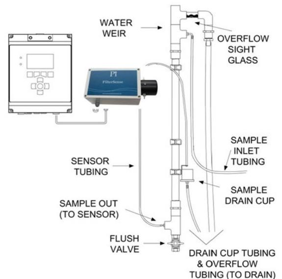
**CRUIS® FilterSense with overflow weir**
